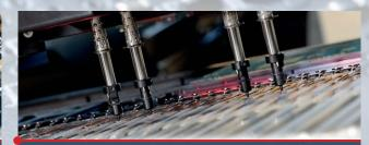
Multi flexible feeder, multi lane cassette or highly accurate single lane feeder. Tape, Stick, Strip, Tray slider. Largest component spectrum; 01005 up to 80 x 80 mm, component height up to 25 mm.
